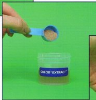
Add sample to CHLOR*EXTRACT and shake for 2 minutes
