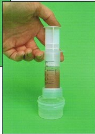
Filter out solids and test with titrator tube
